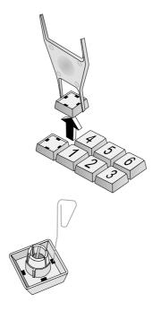
Now remove this key from the keyboard by pulling upwards.
